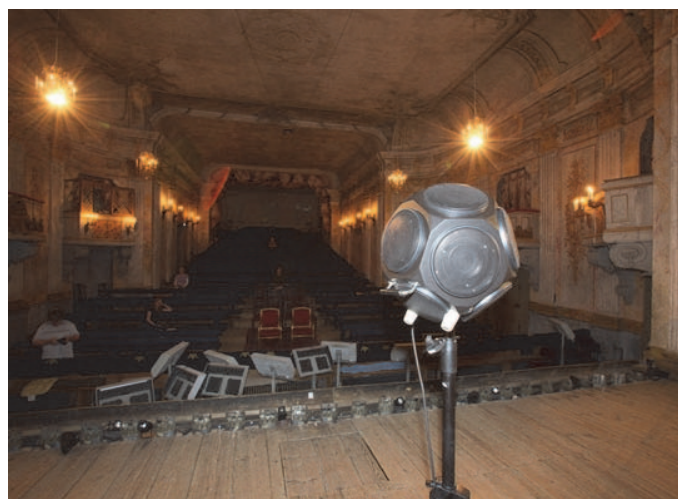
Figure 5. comparison of the reverberation time measured in two theatres (right) and picture from the measurements in situ (left).
