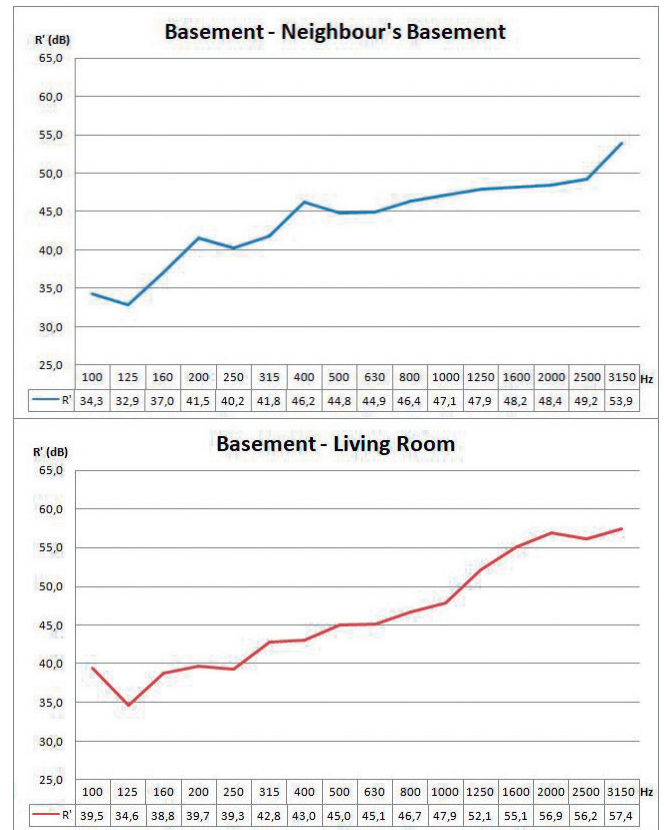
Figure 7. Current insulation level of the wall and the ceiling.
